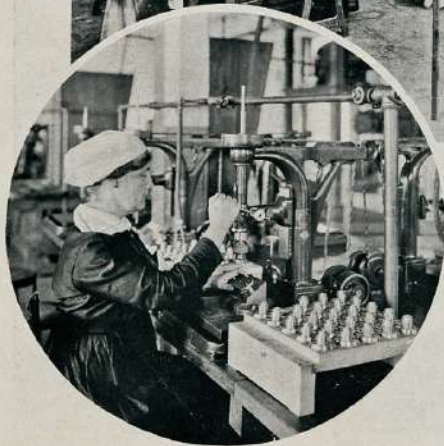
Drilling the Flash Hole No. 80 Fuse
