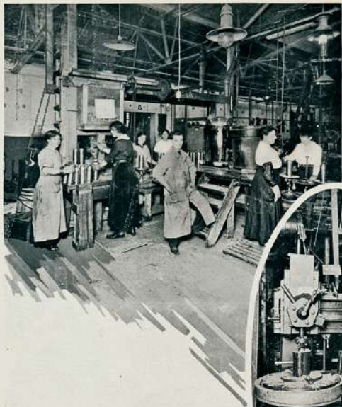
Screwing in and Rough Turning the Brass Socket.
