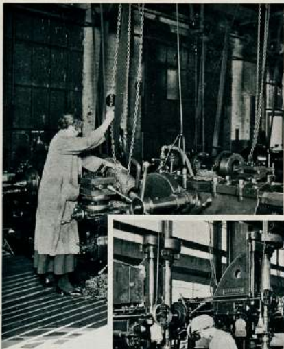
Handling an 8-inch Shell Body with Lifting Tackle Previous to an Operation
