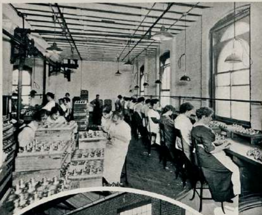
Inspection of Bodies No. 100 Fuse
