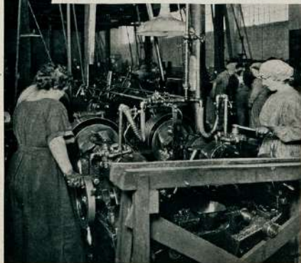
Threading and Chasing Adaptor Thread
