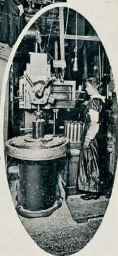
Screwing in and Rough Turning the Brass Socket.
