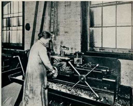
Turning Copper Driving Band
