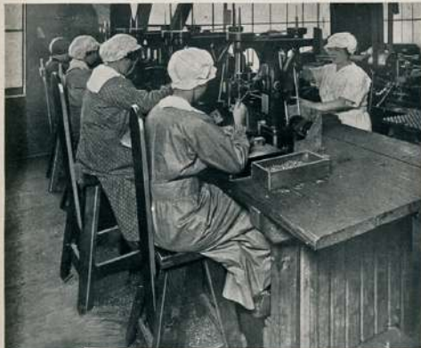
Various Drilling Operations of Small Parts No. 100 Fuse
