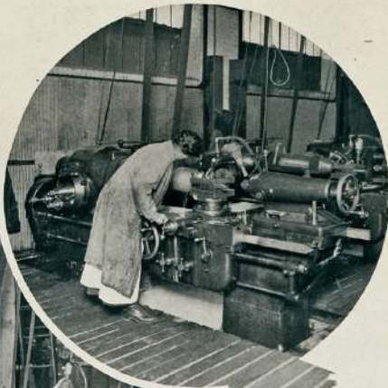
Boring the Fuse Hole 8-inch Shell
