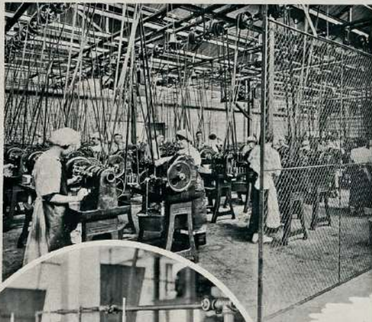
Routing Powder Groove No. 80 Fuse
