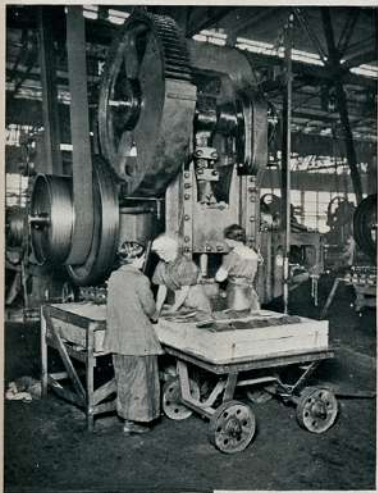
Close View of the Two First Operations of Stamping Cartridge Cases for 18 Pounders
