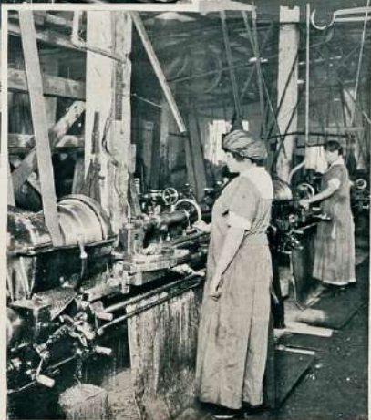
Finish Turning and Profile 4.5 High Explosive Shells
