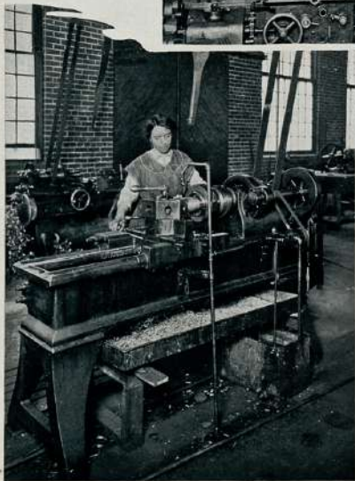
Undercutting the Nose and Cutting Crimping Groove, 18-pounder Shrapnel
