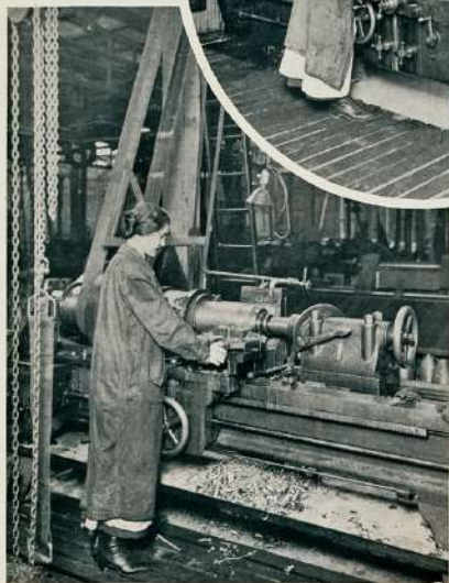
Undercutting and Waving of 8 inch Shells
